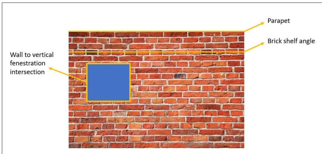
Figure 5. Location of Thermal Bridging
